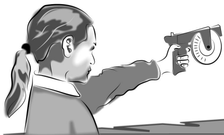
Anna uses a clinometer to measure the angle.
